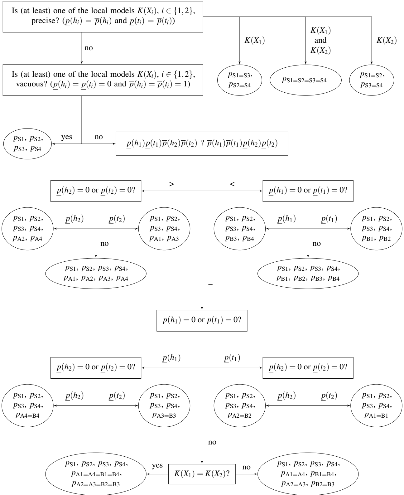
Figure 1: Diagram to obtain the extreme points of the independent natural extension of two binary variables
